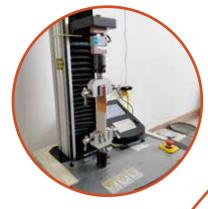
TENSILE STRENGTH TEST
